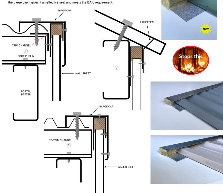
Cut wall sheet approximately 10mm shorter than the top of the roof sheet profile, then install the Barge B.A.L Flashing over cut ends of wall sheet and push down to be level with the top of the roof sheet profiles, compressing the rockwool insert. Can cater for approximately 20mm of variances.
